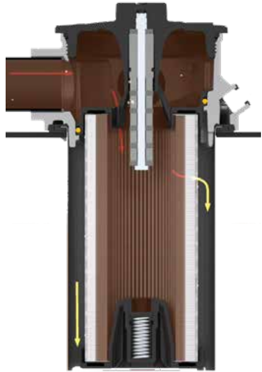
Magnetic pre-filtration and in-to-out filtration
